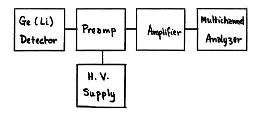
Figure VIII-1. Electronic Block Diagram for Ge(Li) Gamma Ray Spectrometer.
