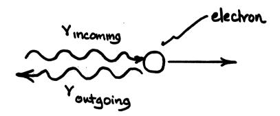
(b) The backscatter peak which corresponds to the  $\gamma$ -ray energy associated with the outgoing photon in a  $180^{\circ}$  scattering as shown
