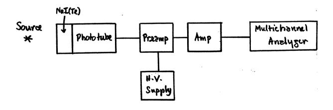
Figure VI-l Electronic Block Diagram for NaI(Tl) Gamma Ray :Spectrometer.
