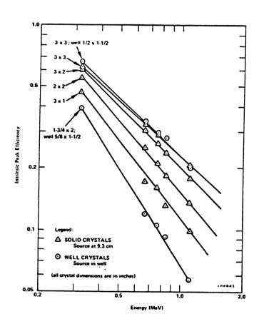
Figure VI-5 Intrinsic Peak Efficiency of Various NaI(T1) Crystals vs. Gamma Energy.
