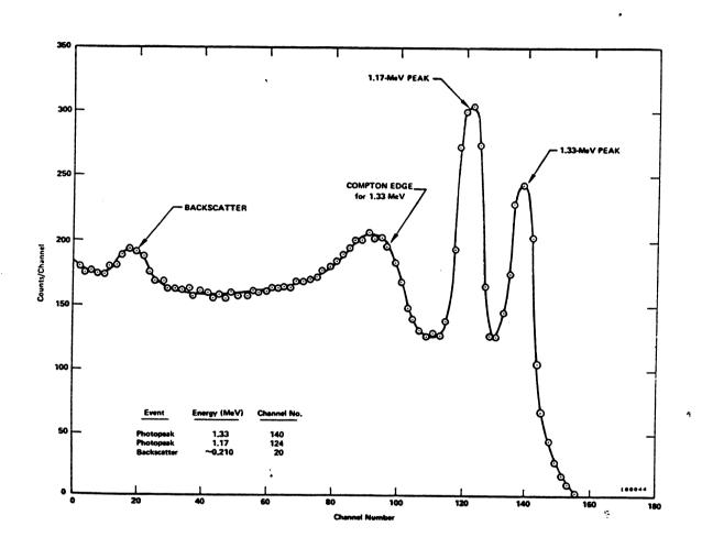
Figure VI-3  $^{60}$ Co pulse height spectrum.
