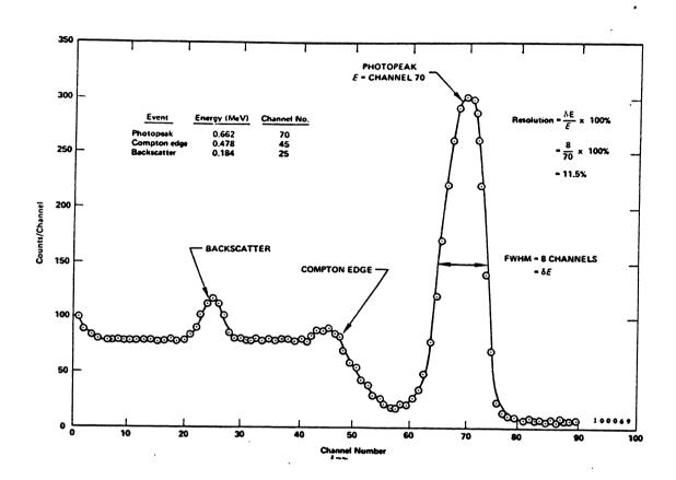
Figure VI-2 A typical <sup>137</sup>Cs pulse height spectrum.
